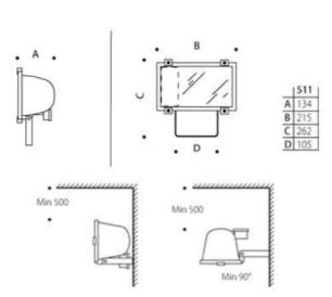
SPIDER tungsten halogen fittings 500W are ideal for security lighting where instant (hot re-strike) is required, or for small area low usage lighting.
